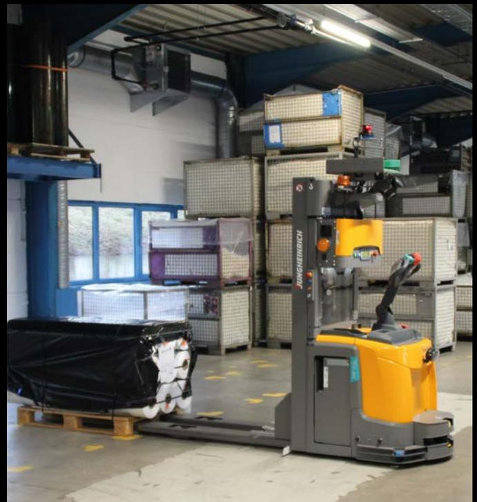
Recurring tasks in warehouse operations are completed fully automatically by the **AGV**.
