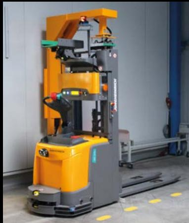
**ERC 215a** with lithium-ion technology and automatic charging – lack of battery replacement saves time and costs.
