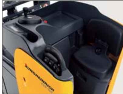
Ergonomic arrangement of operator space on ESD 120
