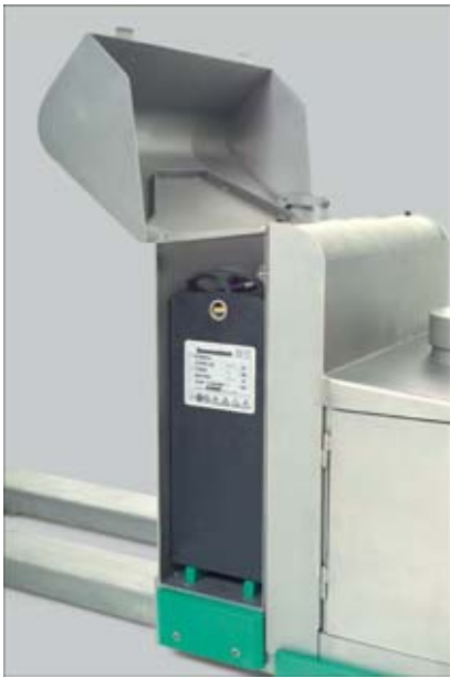
Ready for battery change: open battery cover and removed side panel
