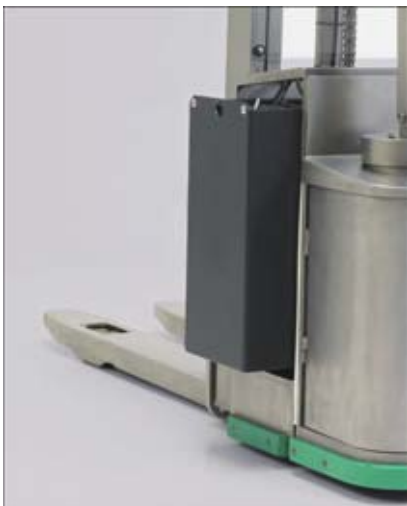
Ready for battery changing: open battery cover and remove side panel
